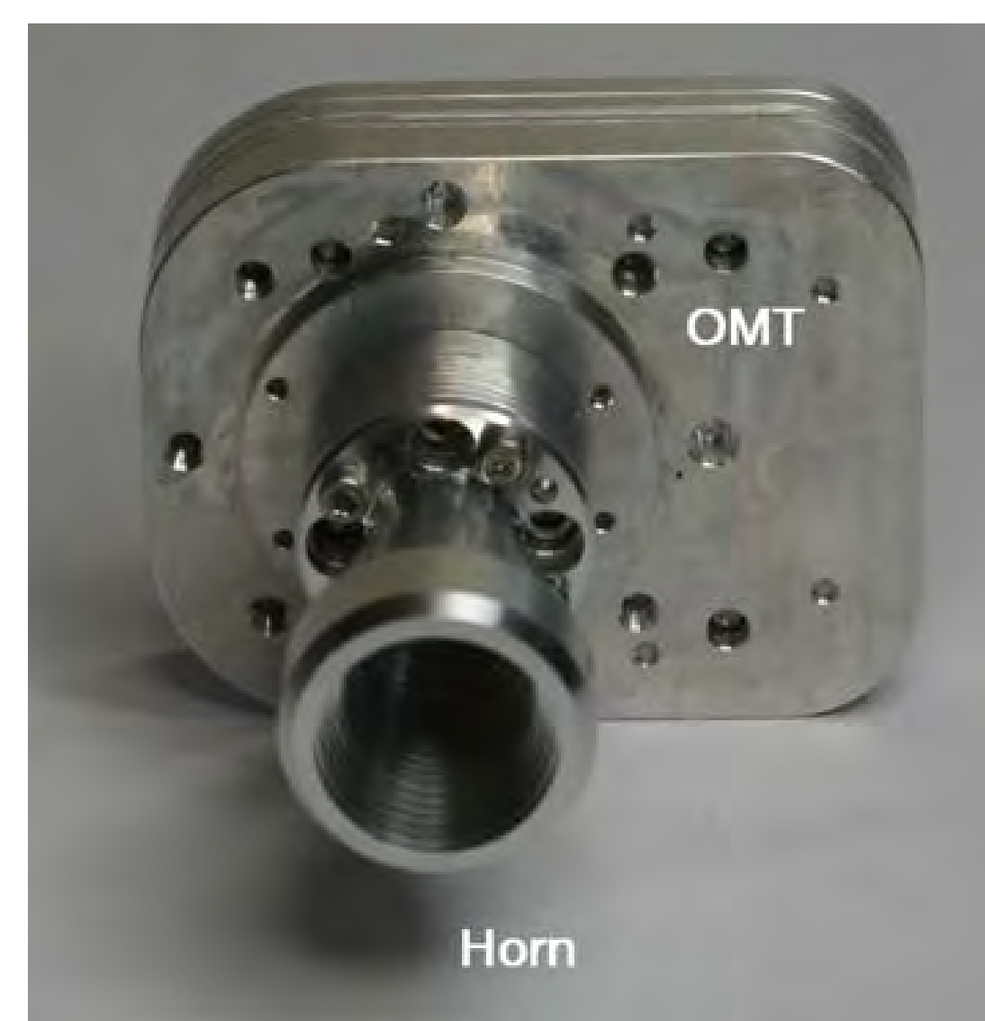
Figure 3: Constructed horn and OMT.
