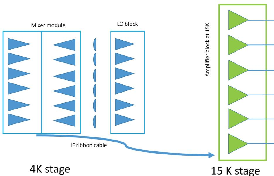
Principle array layout based on building block above which allows to resolve major thermal and element placement problems. Especially IF amplifiers can be placed far away without affecting temperature of mixer module. The array can be built out single pixel mixer modules that can be tested separately to retain state of art performance. Current estimate that 128 pixel array in this configuration is feasible to build.
