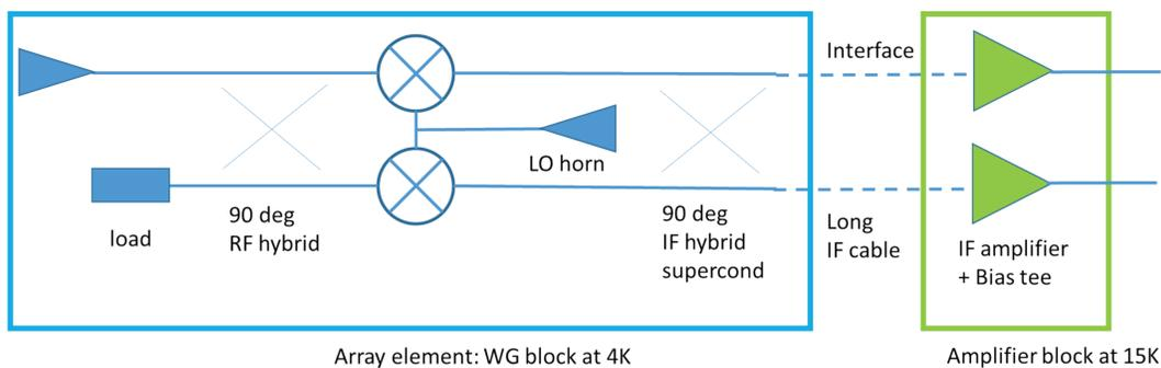
Principle mixer layout realized for ALMA band 9 2SB upgrade project and SEPIA 650 GHz channel at APEX telescope. Note absence of cryogenic isolator. This makes it possible to expand IF bandwidth to 32 GHz in this system (Measured is 3-12 GHz IF band). IF amplifiers can be located far from mixer and can even be on different temperature level, which is important for focal plane array implementation
