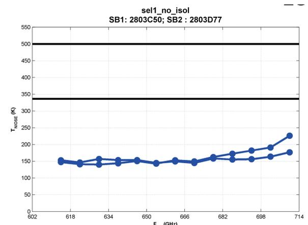
Measured SSB noise temperature. USB and LSB curves. Temperature is averaged over 4-12 GHz IF band.
