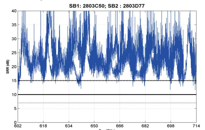
Measured sideband ratio of the system. Note that average level of SBR is about 15dB which allows to reduce system noise
