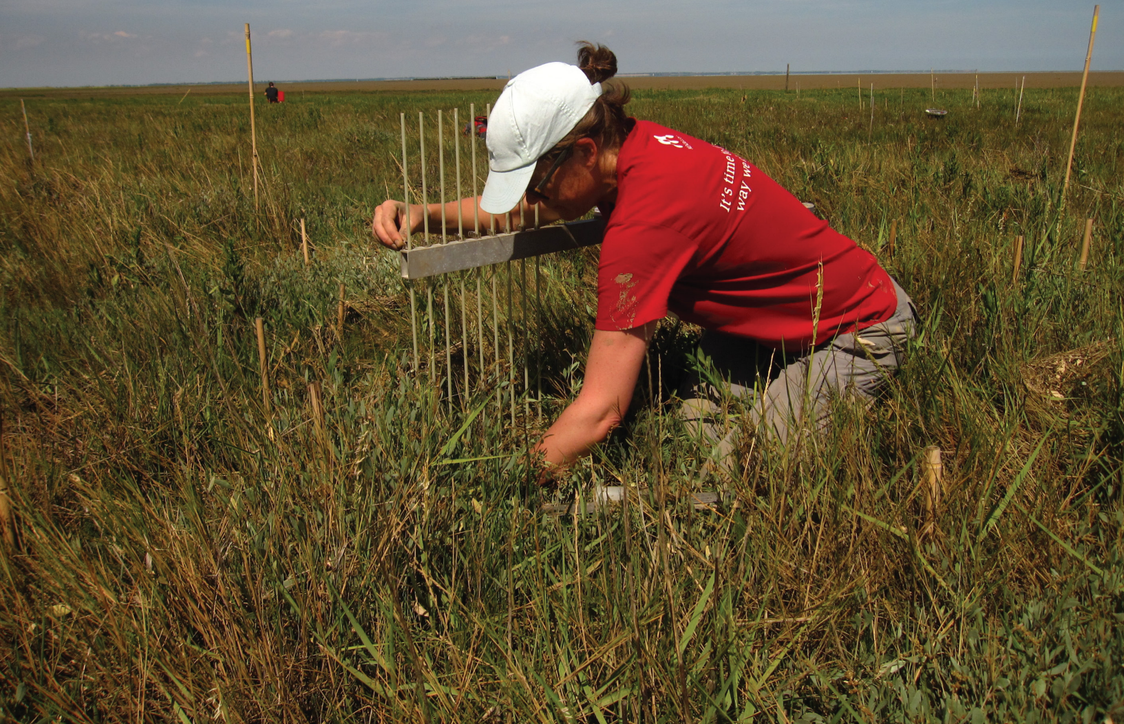
Figure 15. Measuring elevation change using a Sedimentation-Erosion-Table (SET) at Tillingham, UK (photo: M Yates)
