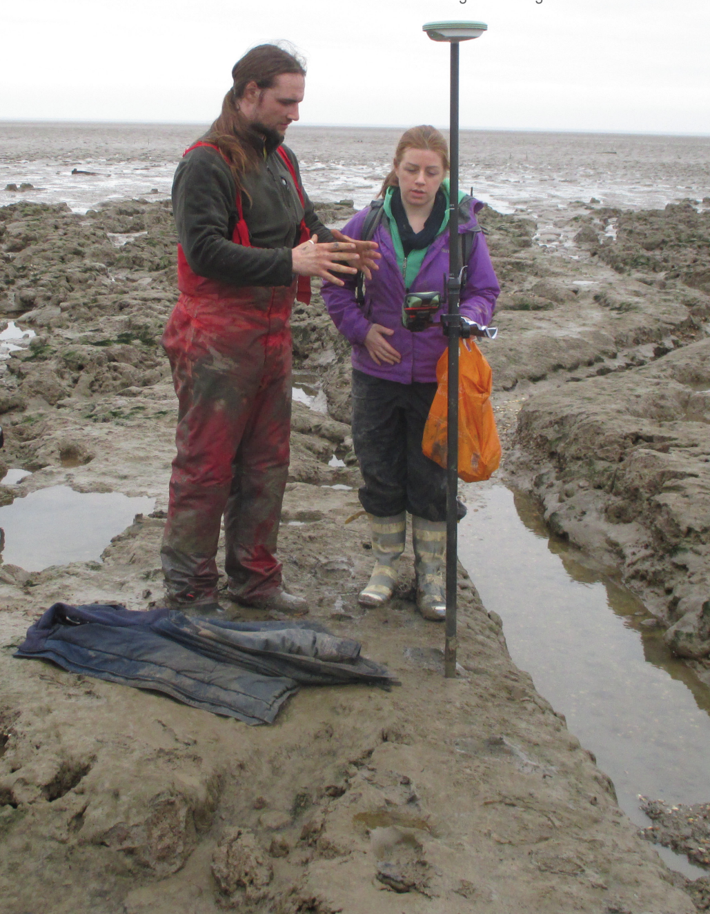
Figure 8. Use of differential Global Positioning Systems (dGPS) for accurate coordinate and height determination of all measurement plots and instrumentation (photo: I Möller)
