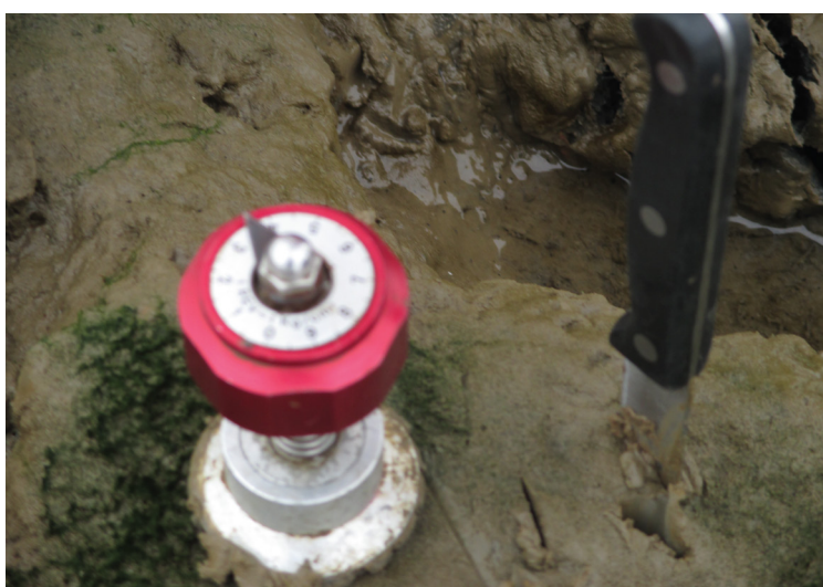
Figure 13. The 'shear vane' instrument for recording the rotational force that needs to be exerted on the top layer of sediment before it fails (photo: I Möller)
