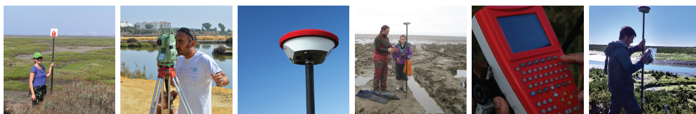
Figure 18. Collecting in situ elevation data at the FAST case study sites. Creators: Edward P. Morris, Jesus Gomez Enri, Juan Carlos Gutierrez, Iris Möller, and Gloria Peralta.
