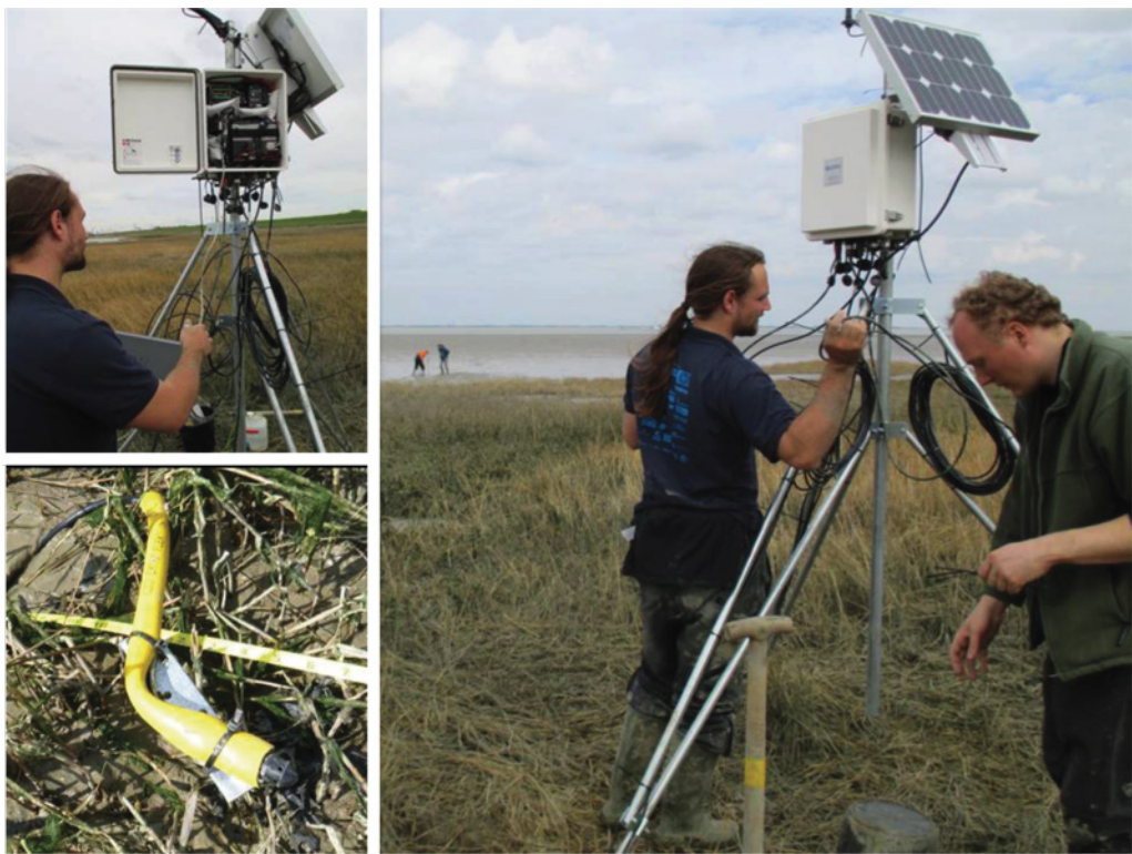
Figure 6. Wave monitoring stations were installed at each of the eight FAST field sites, with wires connecting up to six bottom-mounted pressure sensors (inset bottom left) (photo: I Möller).
