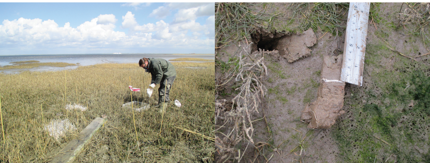
Figure 16. Accretion marker horizons sprinkled onto the marsh surface at the start of the project at Paulinaschor, The Netherlands, and buried marker horizon after two years of deposition at Donna Nook, UK (right) (photo: I. Möller)
