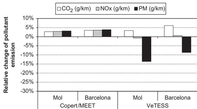
**Fig. 3.** Relative change between the emissions of two urban driving cycles (30 kph limit relative to 50 kph limit), driven with a Citroen Jumper diesel LDV (Mol, Cycle 5: 18.9- > 18.3 kph; Barcelona, Cycle 2: 14.5- > 13.9 kph; see Table 1 for details).
