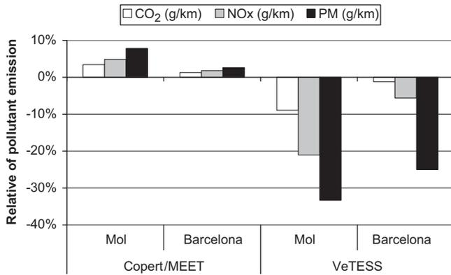
**Fig. 2.** Relative change between the emissions of two urban driving cycles (30 kph limit relative to 50 kph limit), driven with a Skoda Octavia passenger car (Mol, Cycle 4: 25.2- > 22.7 kph; Barcelona, Cycle 1: 14.8- > 13.9 kph; see Table 1 for details).
