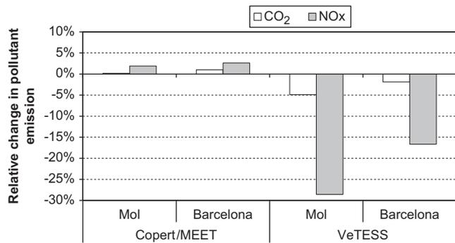
**Fig. 4.** Relative change between the emissions of two urban driving cycles (30 kph limit relative to 50 kph limit), driven with a VW Polo petrol passenger car (Mol, Cycle 6: 21.8- > 20.3 kph; Barcelona, Cycle 3: 17.8- > 15.9 kph; see Table 1 for details).
