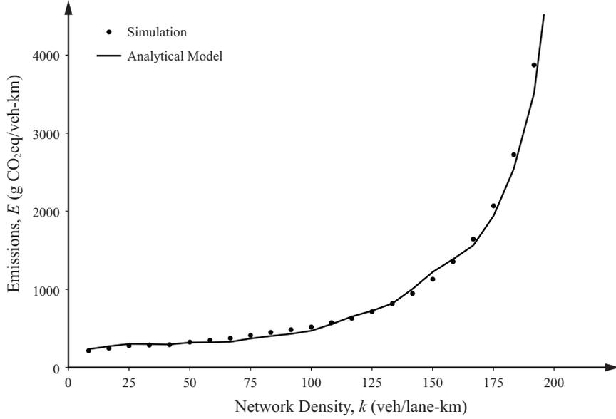
Figure 4. Network-wide emissions estimated using an analytical model based on the MFD and estimated using detailed trajectories from a simulation and microscopic emission analysis ( $G/C = 0.50$ ;  $C = 60$  sec;  $\ell = 0.30$  km).
