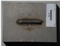
Inconel GTAW welded plates ( NeT project )
