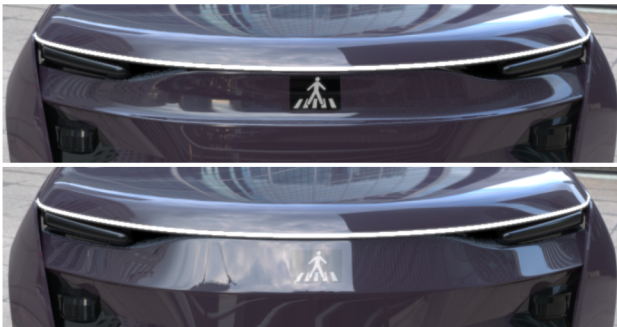
Figure 18: impact of outer lens inclination on contrast and required Brightness
