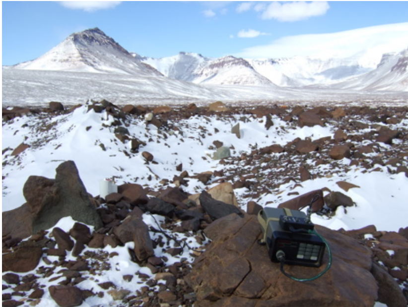
Figure 3.7: Magnetometer base station in Beacon Valley, 25 m from the camp. The white-painted sensor is to the left of centre.
