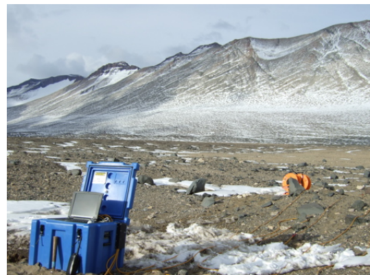
(d) The console, battery and recording laptop for the two-dimensional resistivity tomography.
