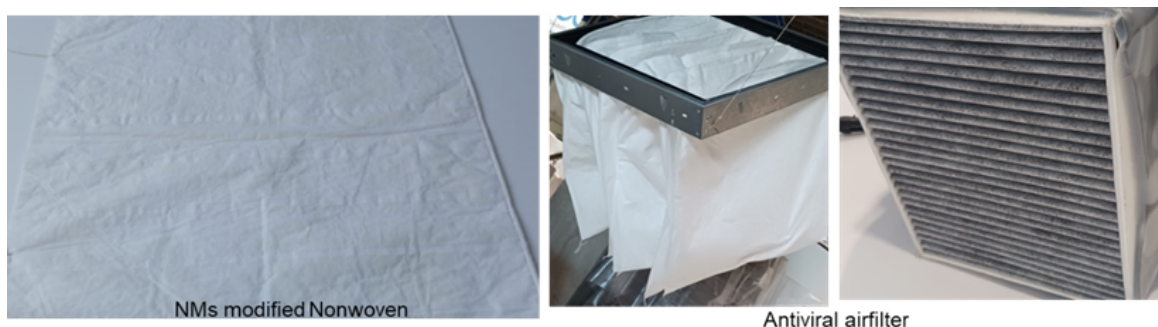
Figure 4.2.1: Nonwoven materials activated with antiviral MNs before and after their mounting in filter frames.
