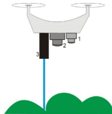
Figure 1. Drone-based technique used to record the fluorescence of plants under the remote laser excitation.
