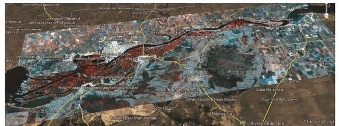
Figure 1. An example of dual-use GEOINT product; change detection of the Sentinel-1 satellite Synthetic Aperture Radar (SAR) imagery after demolition of the Novaja Kahovka dam on June 6, 2023, scattering coefficient difference shows flooded areas (red), two SAR-s were compared (Google Maps as the base layer).
