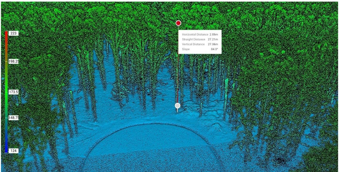
Figure 4. 3D model of an old oak stand taken by a DJI R300 drone equipped with an airborne LiDAR head, generated from a point cloud with a graduated symbology of the height above sea level (courtesy of "Croatian Forests" Ltd.).
