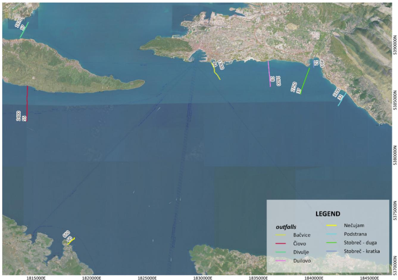
Figure 2. Marine Outfalls in the wider aquatorium of Split. The first number is the length of the pipe, and the second is the depth of the discharge point (expressed in meters).
