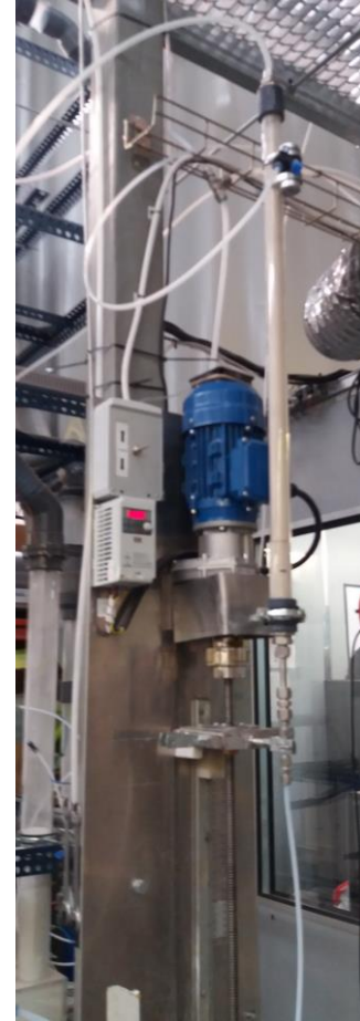
Figure 2.7 Scheme of the solid feeding system used in most the carbonation test in entrained mode (gas and solids moving downwards).
