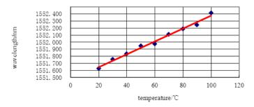
Figure 20. The wavelength - temperature diagram of FBG3
