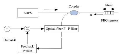
Figure 5. Scanning optical fiber F - P interference detection
