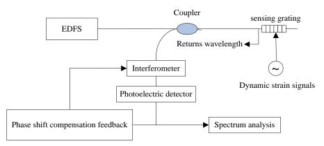
Figure 4. Non-equilibrium fiber M - Z interference detection
