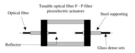
Figure6. The structure of FFP
