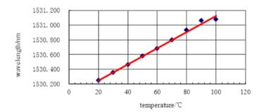
The relationship between temperature and center wavelength of FBG1 is shown in figure 18.
