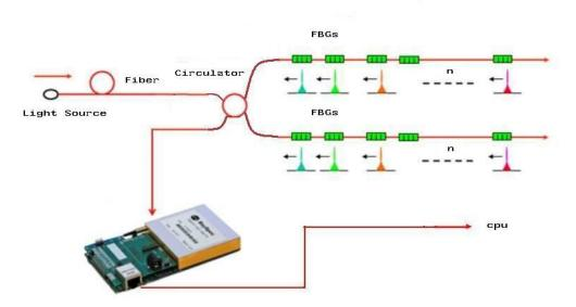
Figure 8.The diagram of fiber Bragg grating temperature sensor
