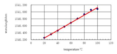
Figure 19. The wavelength - temperature diagram of FBG2
