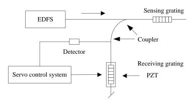
Figure3. Matched fiber grating detection method
