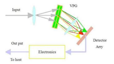
Figure 7. Schematic diagram for FBG Analyzer module
