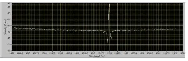
Figure14. Single FBG wavelength-power of the XY graph
