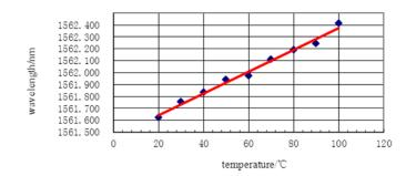
Figure 21. The wavelength - temperature diagram of FBG4
