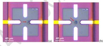
Fig. 1. Individual biological cell handling and trapping at UHF frequencies respectively in (a) positive and (b) negative DEP configuration.
