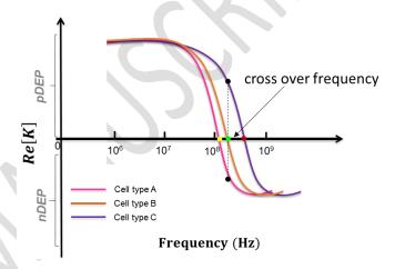
Fig. 3. Potential effect of intracellular dielectric specificities on the Claussius-Mossotti factor for various biological cell types (schematic view).
