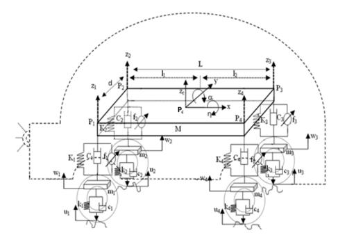
Figure 5 Full vehicle nonlinear active suspension systems
