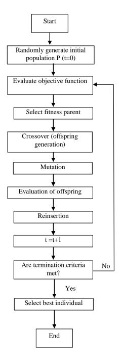
Figure 3. Structure of an evolutionary algorithm
