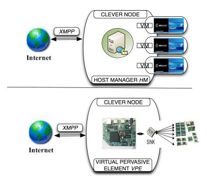
Fig. 8. CLEVER node: on the top side the original version aimed at Cloud Technology. On the bottom side the modified version able to support more type of Sensing Technology.
