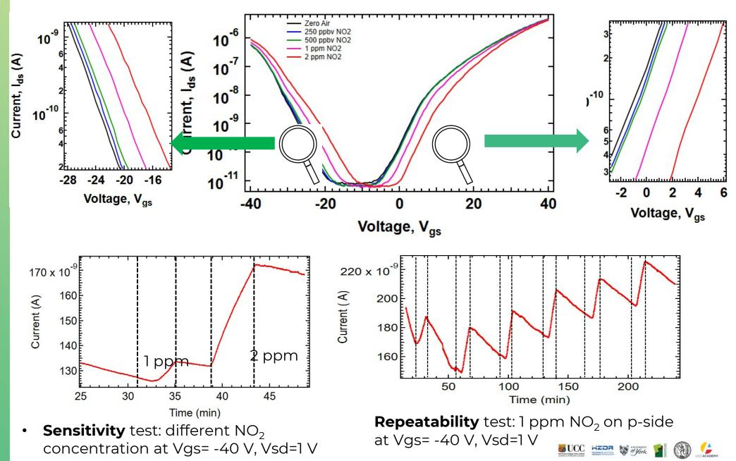
Si-JNT: Sensing NO<sub>2</sub> at sub-ppm level
