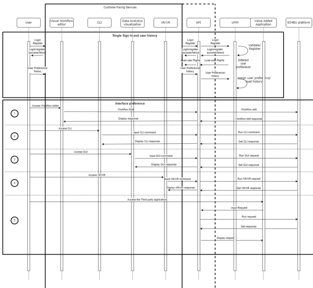
Figure 28 Customer Facing Services - Sequence Diagram
