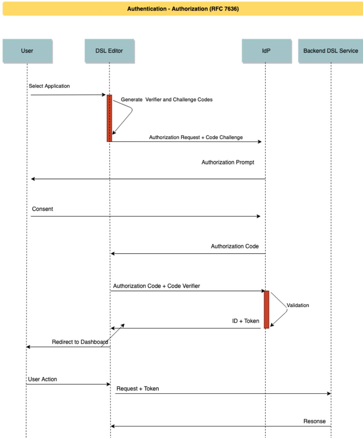
Figure 26 DSL Engine Authentication
