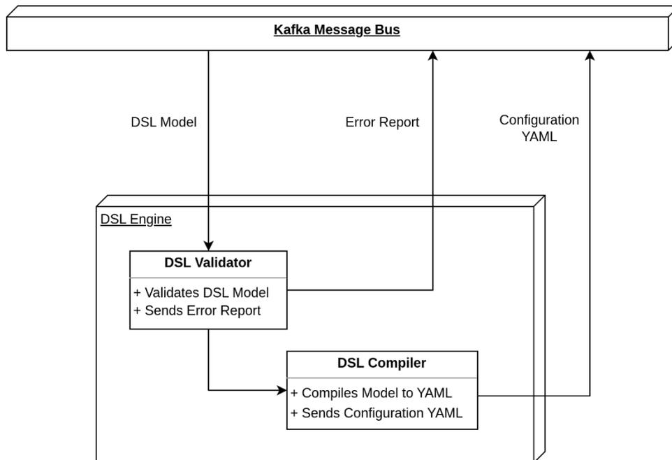
Figure 9 DSL Engine Class Diagram
