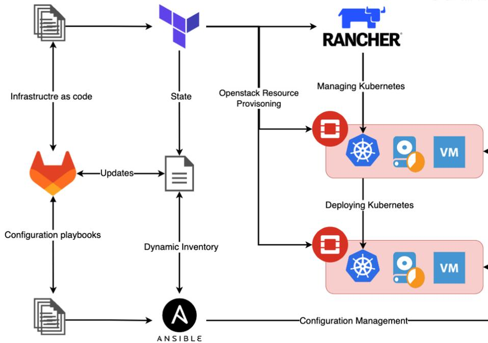
Figure 4 IaC and GitOps Pipeline Design
