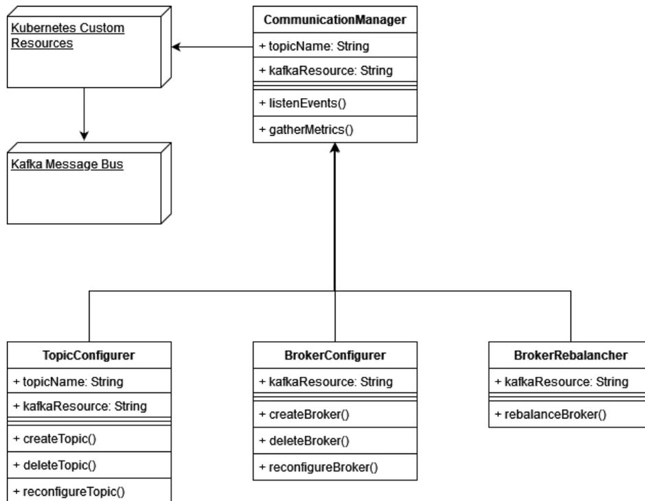
Figure 8 Communication Manager Class Diagram
