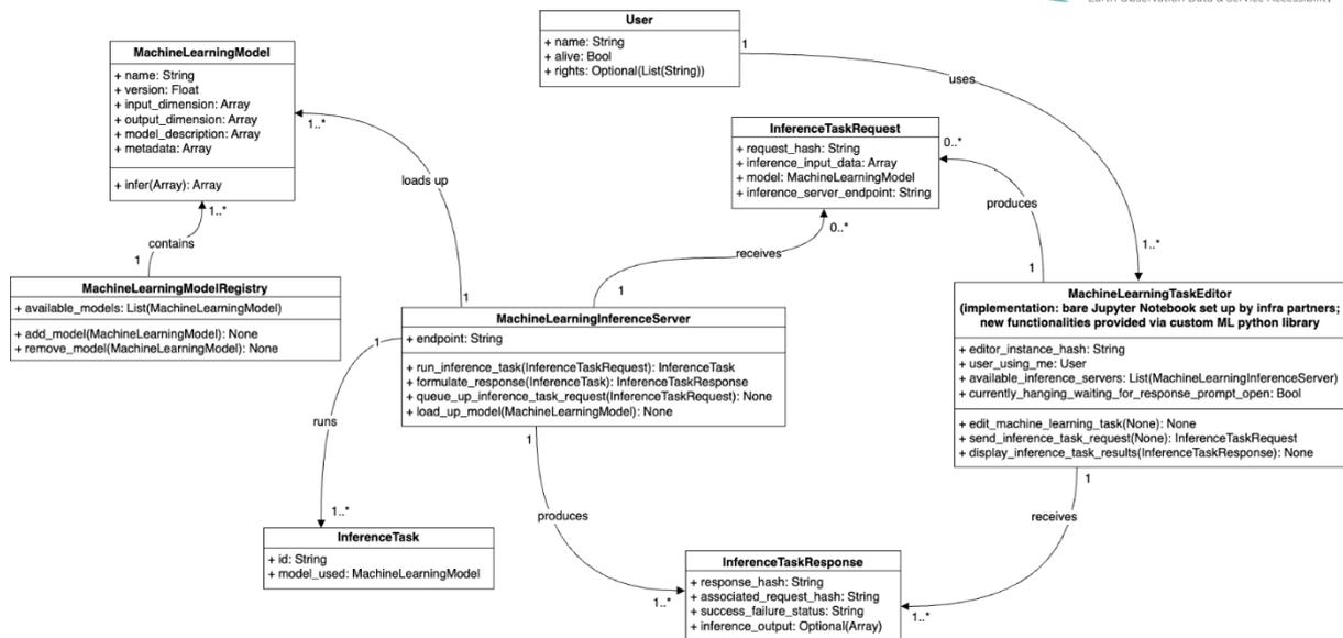
Class diagram of the integration of the ML component
