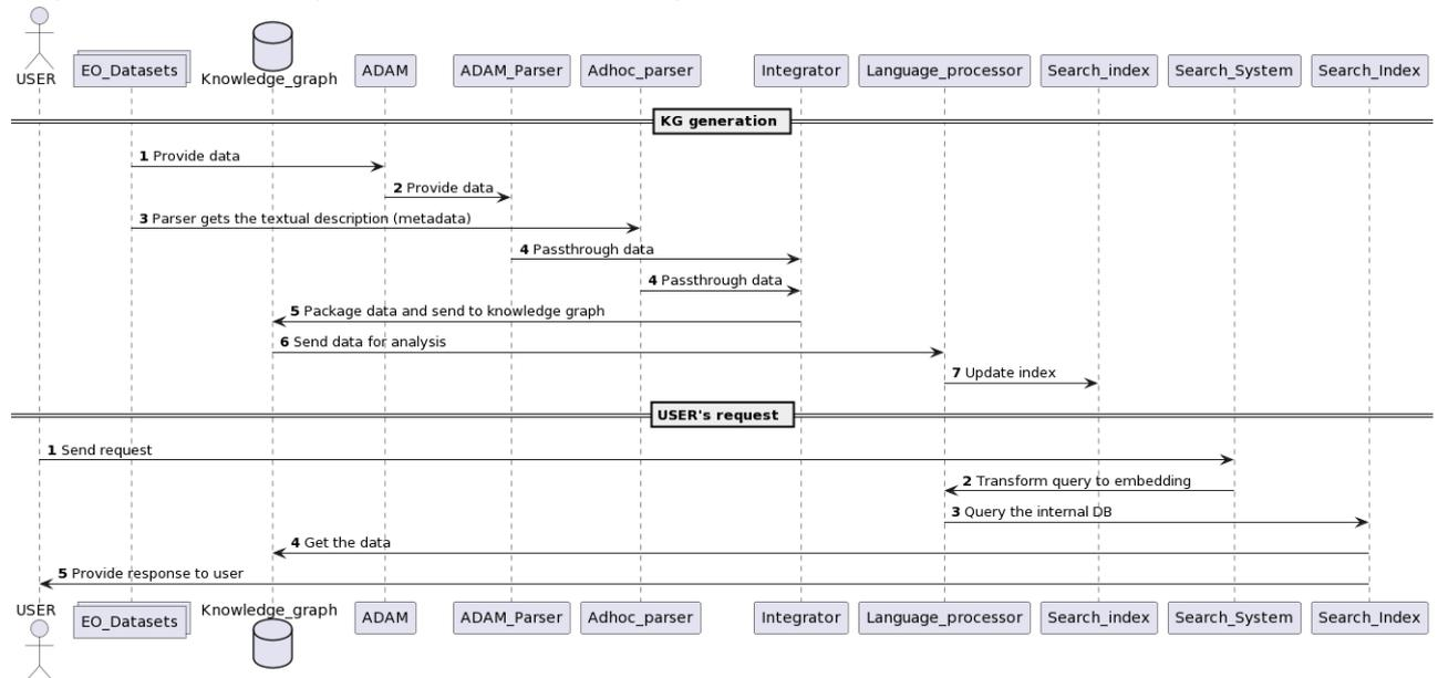
Figure 19 - KG Sequence Diagram
