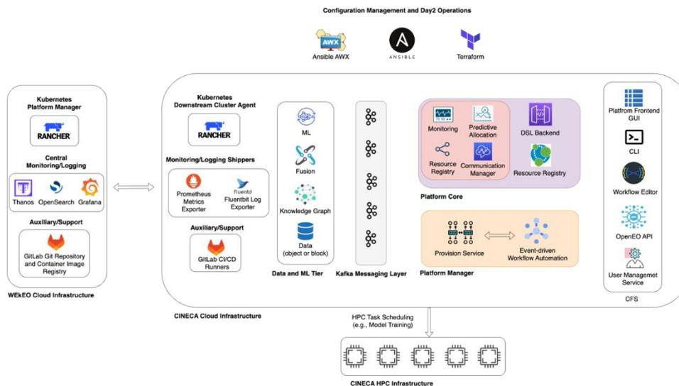
Figure 5 EO4EU Multi-cloud Infrastructure High-level Design
