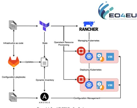
Figure 4 IaC and GitOPS Pipeline Design
