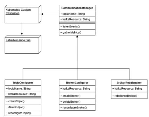
Figure 8 Communication Manager Class Diagram
