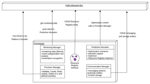
Figure 7 Platform Orchestrator Class Diagram
