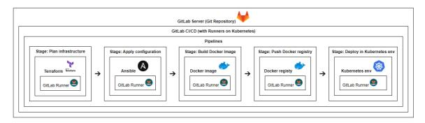
Figure 6 Continuous integration general schema
