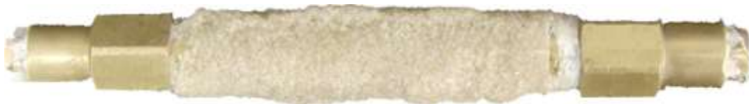
Figure 9: Air hammer for inducing shear waves in model
