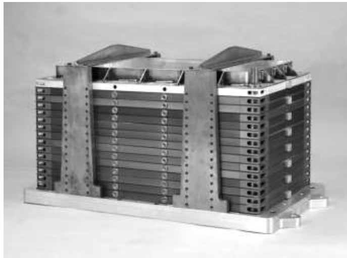
Figure 13: A view of the IFSTTAR ESB Box (note that the top ring made of steel sheets is only made for the pluviation process and is removed in operation)
