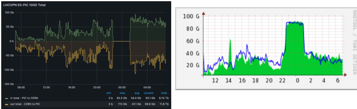
Figure 6.8b: Two plots showing successful activation of NOTED at PIC, operating as a DEMO site, to implement load balancing between LHCOPN and LHCONE from February 21st to 23rd, 2024.
