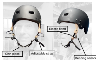
Figure 1. MARRYS helmet for mechanical measure of lower jaw displacement.
