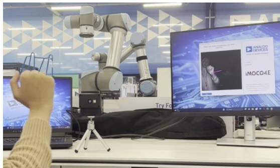
Figure 2. Wrist Tracking in the Teleoperation system.
