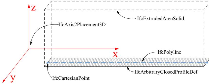
Figure 6: Main IFC classes used to create a geometric representation of the wall (Zbirovský, 2024).
