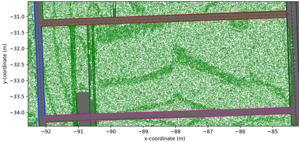
Figure 4: Walls (colored) segmented from point cloud (green), represented with their axes (Zbirovský, 2024).
