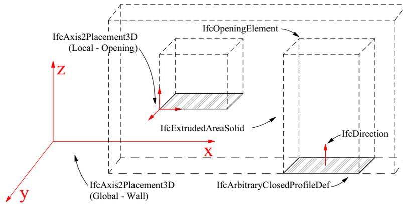
Figure 7: Main IFC classes used to create a geometric representation of opening. (Zbirovský, 2024).
