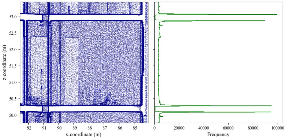
Figure 3: Point cloud cross-section (on the left). A z-coordinate histogram of point cloud data (on the right) (Zbirovský, 2024).
