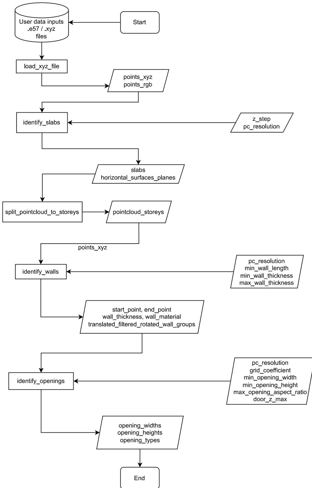
Figure 2: Program flowchart illustrating the algorithm for converting unorganized point clouds into a digital model of a building. The flowchart depicts the code implementation's inputs, outputs, and sequential steps.
