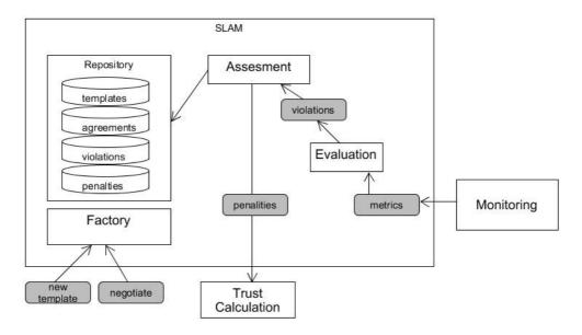
Figure 11. Component diagram of SLA Manager (SLAM)
