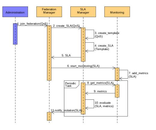
Figure 12 Sequence diagram of the SLA lifecycle
