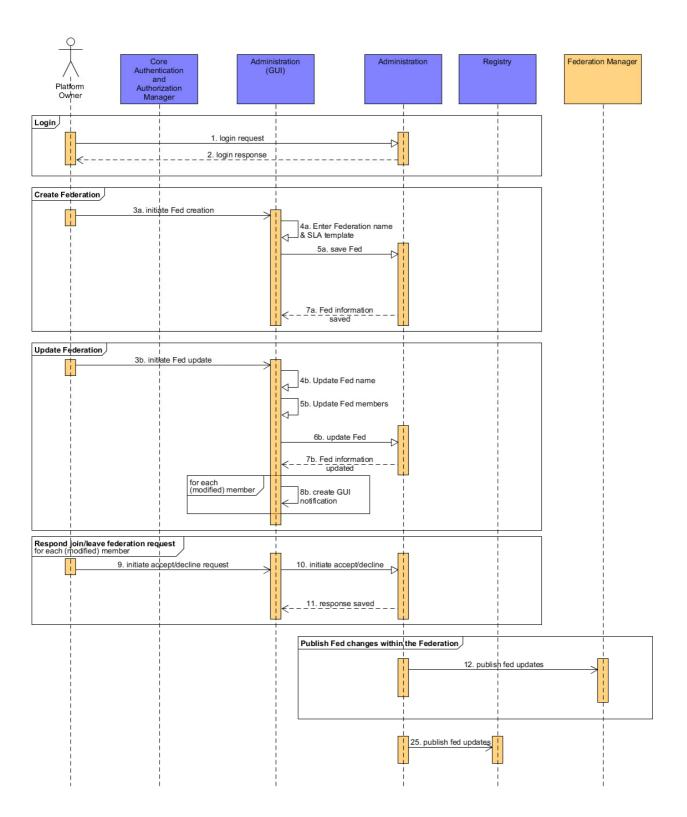
Figure 7. Manage (Create, Join and Leave) federations – Core Domain interaction
