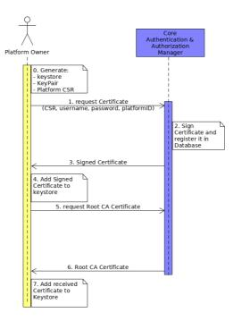
Figure 25 Sequence Diagram of intermediate CA certificate acquisition
