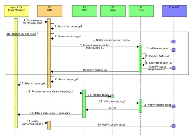
Figure 20. Sequence diagram of Bartering
