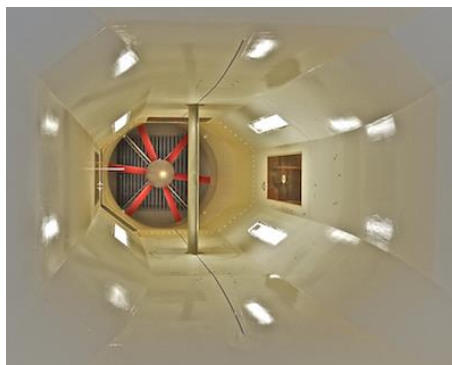
Figure 1. Test section view of Glasgow Hanley Page Tunnel
