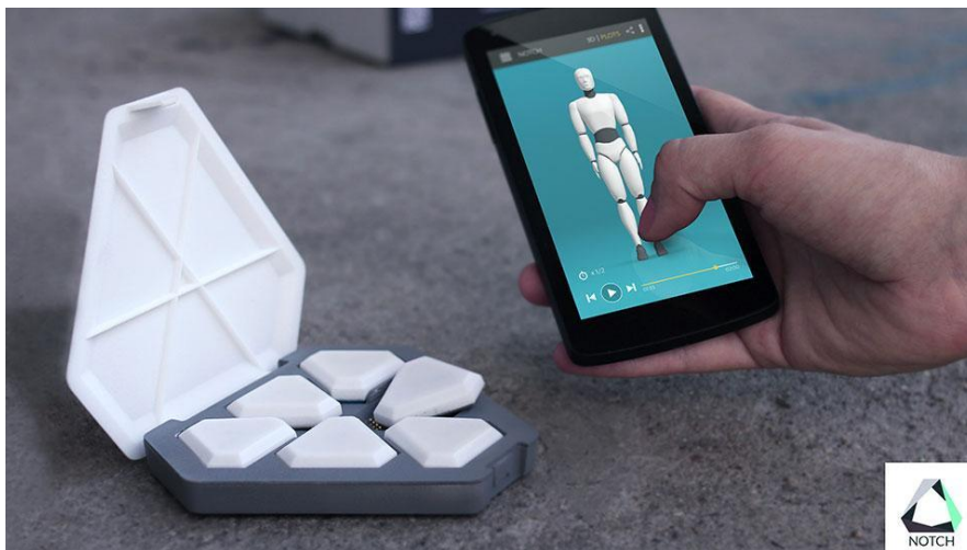
Figure 4. A set of six notch sensors that allows upper body tracking
