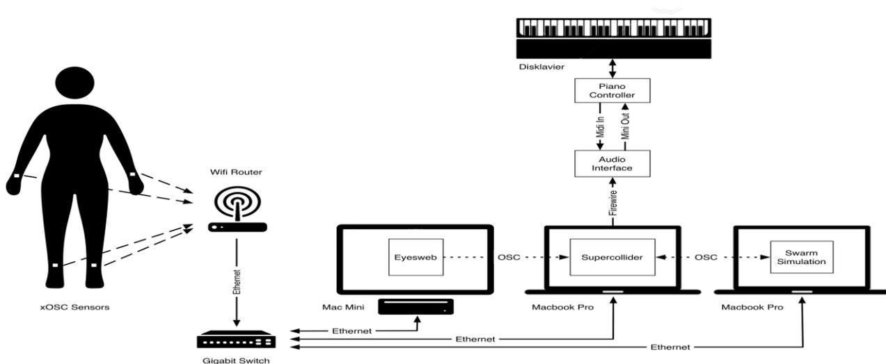
Figure 5-2. Schematic Depiction of Technical Integration of the Sensing, Communication, Computation and Piano Control
