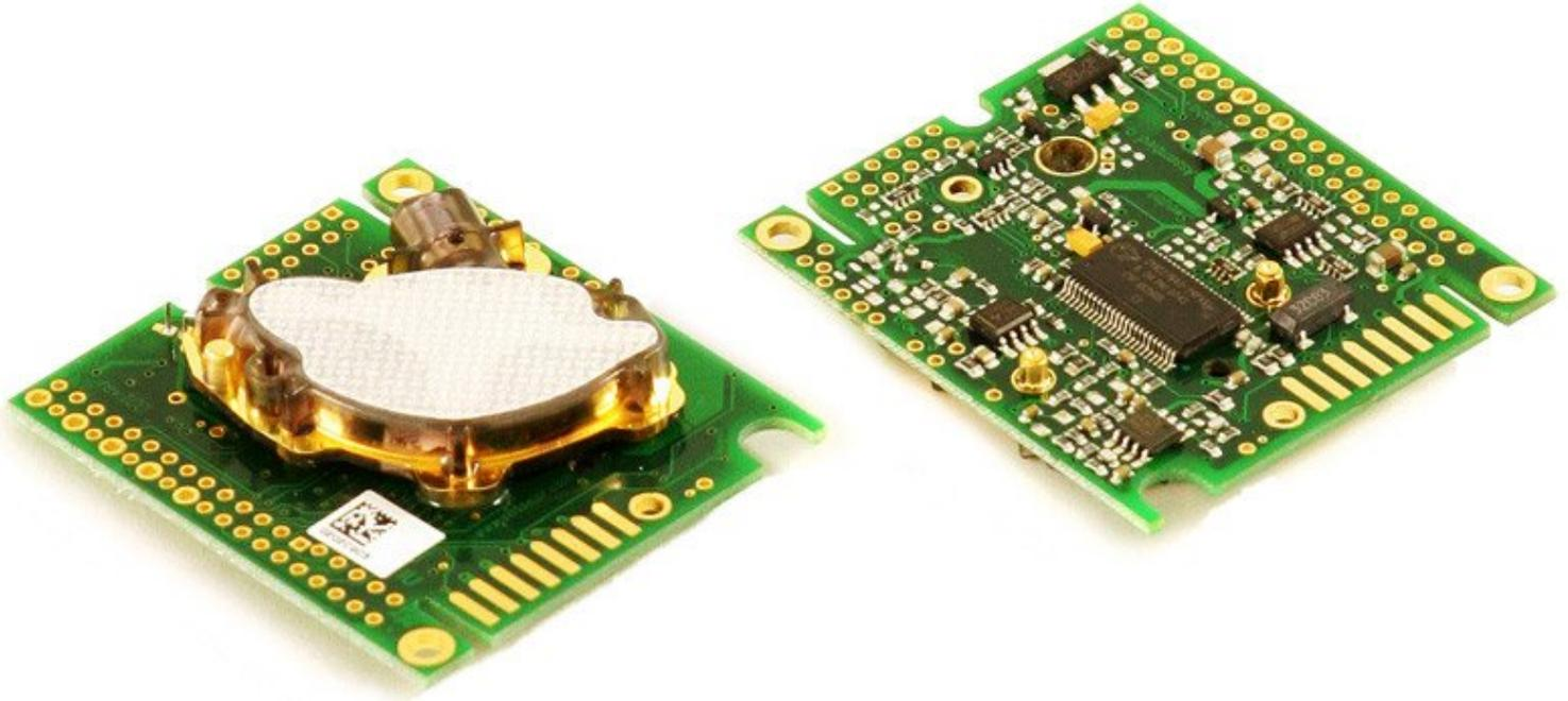
Be very careful when connecting the K-30, as there is no reverse-voltage protection and improper connections could destroy your sensor.
