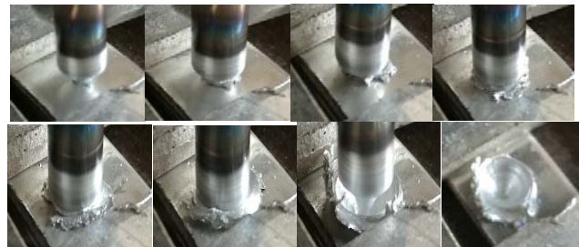
Fig. 8 Sequence of FSSW for AA1100
