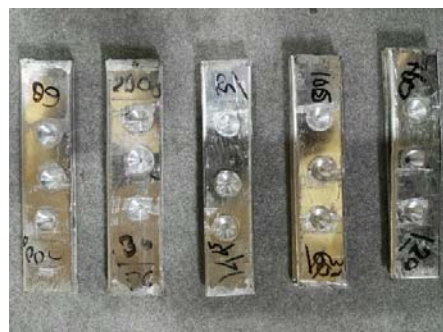
Fig. 11 Surface flash removal
