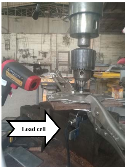
Fig. 6 Load cell and infrared temperature device arrangement
