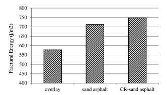
Fig. 4 Fractural energy for three asphalt mixtures
