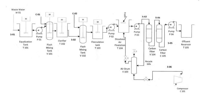
According to (figure 1) the effluent wastewater first process in a clarifier and DAF (Dissolved Air Floatation) for the removal of oil and other impurities as illustrated in (Table 2).
