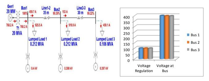
Figure 03: Simulation in ETAP without solar power.
