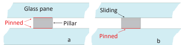
Fig. 3 Simulation conditions for support pillars: (a) top-bottom pinned pillars, and (b) bottom pinned-top sliding pillar
