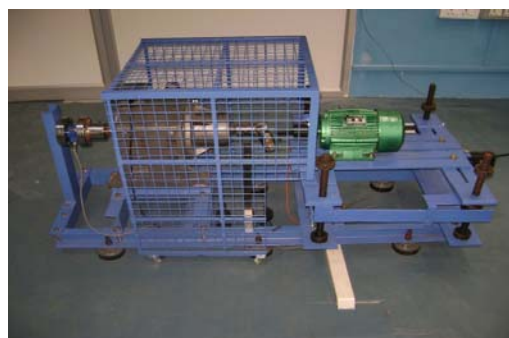
Fig. 7 View of the Motor Test Bed - 1 with 5 HP Motor installed
