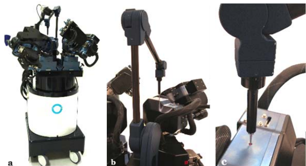
Fig. 1 (a) The neuroArm manipulator is being registered using a registration system, (b) Configuration of the digitizing arm, and (c) Digitizing probe with a ruby spherical tip touches a fiducial marker
