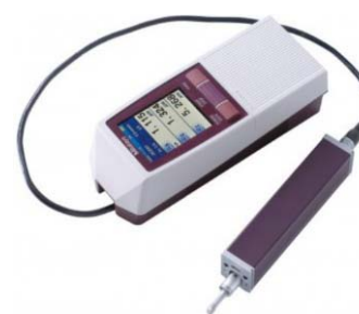
Fig. 3 Roughness meter used to measure surface roughness
