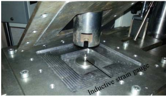
Fig. 2 Experimental setup and section of the test device [10], bottom: inductive strain gauge (ISG)
