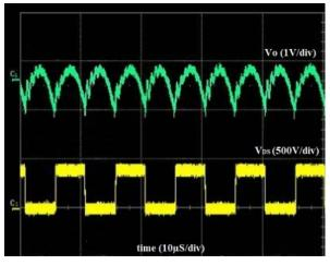
Fig. 16 Output voltage waveform at full load condition
