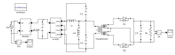
Fig. 4 Simulation circuit for the proposed LLC converter
