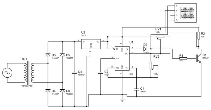
Fig. 12 Pulse generator circuit design using proteus
