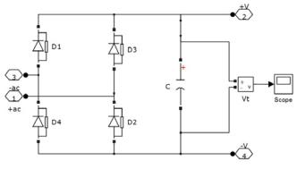
Fig. 5 Simulation of rectifier subsystem block
