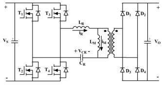
Fig. 1 A full bridge LLC resonant converter
