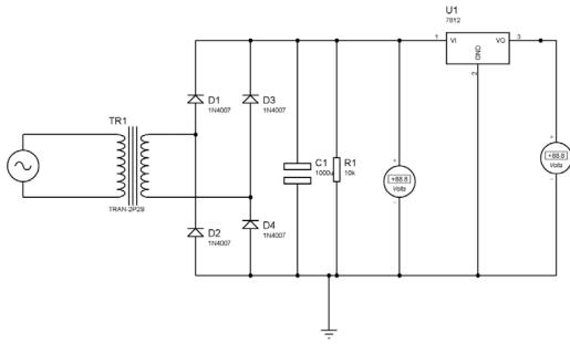
Fig. 11 Rectifier circuit design using proteus
