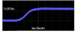
Fig. 17 Output voltage during soft start condition
