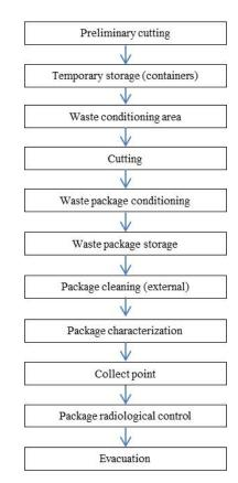
Fig. 2 Flowchart of core dismantling process
