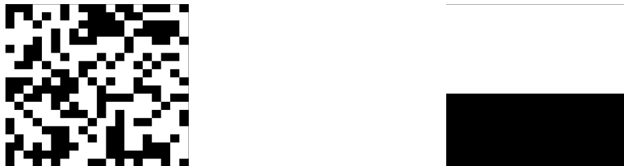
Figure 1: The Random environmental pattern, typically investigated in swarm collective perception research (left). The Stripe pattern, which was explored in our study (right).
