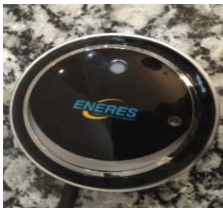
Fig. 3 Indoor temperature, relative humidity and illuminance measuring device
