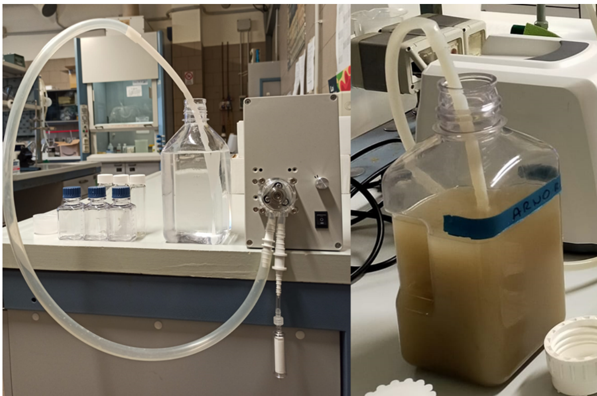
Figure 1: Filtration system with the homemade portable peristaltic pump and Sterivex filter (left panel). Detail of the Teflon tube inside a river sample. (right panel) Credit: Chiara Santinelli
