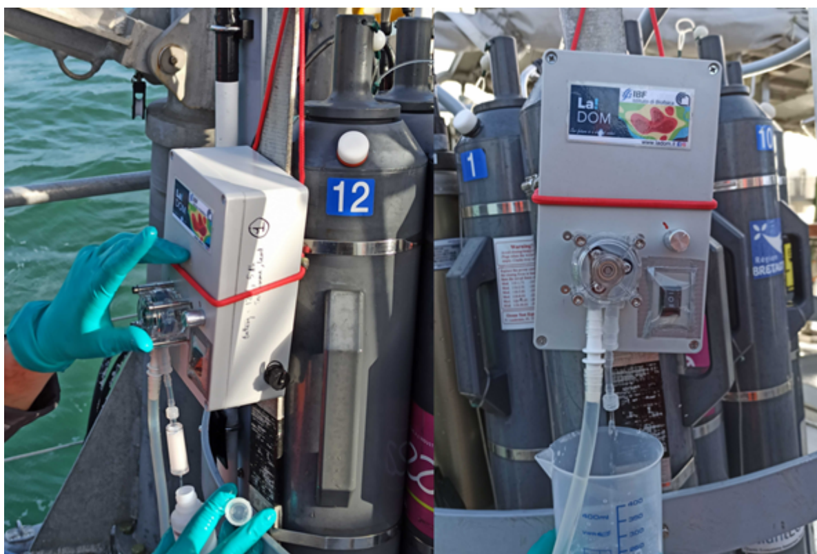
Figure 1. Homemade portable peristaltic pump connected with the Niskin bottle and Sterivex filter.
