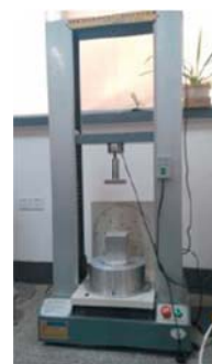
Fig. 3 The test equipment used for the calibration of FTS
