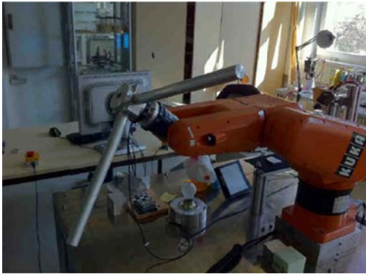
Fig. 4 Realization of the calibration method "Shape from motion": FTS is attached to the load of known weight that rotates by the manipulator along a predetermined trajectory
