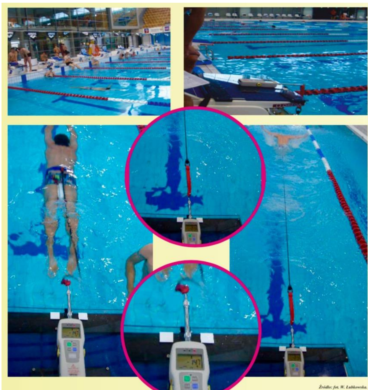
Figure 2. The measuring system used when testing the thrust in the water
