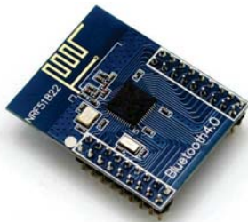
Fig. 7 Minimum working development BLE module nRF51822 SoC
