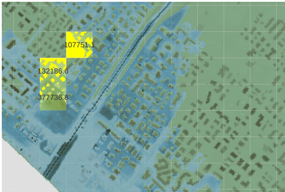
Figure 12: Example of flooding layer and its effect on the buildings in the case of Massa, obtained using exposure vector layers by D6.3 [14]. In this picture, the computed damage (in €) on three selected areas is reported in the related yellow-marked cells, using QGIS software [41].
