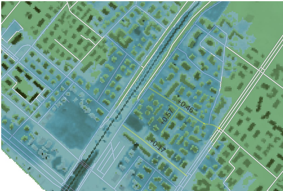
Figure 11: Example of flooding layer and its effect on the road network in the case of Massa, obtained using exposure vector layers extracted from D6.3 [14]. In the picture, the average depth of water (in meters) on some selected roads is shown using QGIS software [41].
