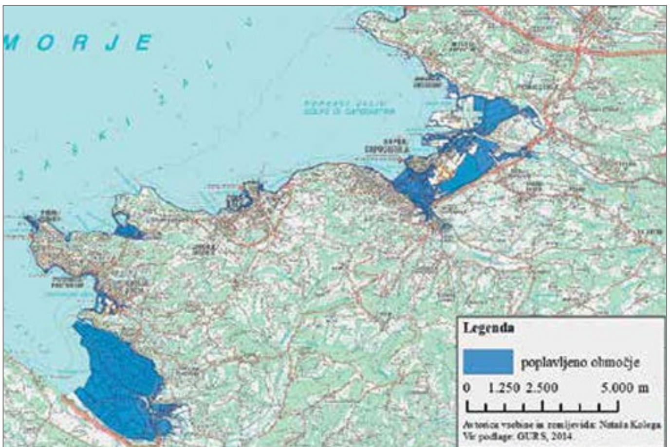
Figure 24: Flooded areas (blue) in case of rising mean sea level by 100 cm and high tide. From: Grubar et al. (2019).
