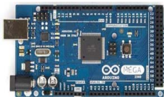
Fig. 3 Model of Arduino Mega 2560 R3 Front [7]
