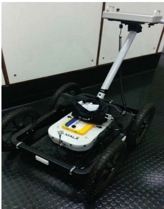
Fig. 1 GPR on a Terraplug Rough Terrain Cart
