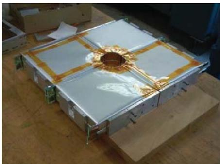
Fig. 2 AD0 detector placed in metal structure
