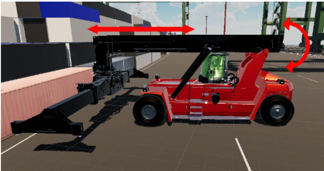
Figure 3.6: “M” and “N” keys are used to extend and retract the boom, while “J” and “K” rotate it up or down.
