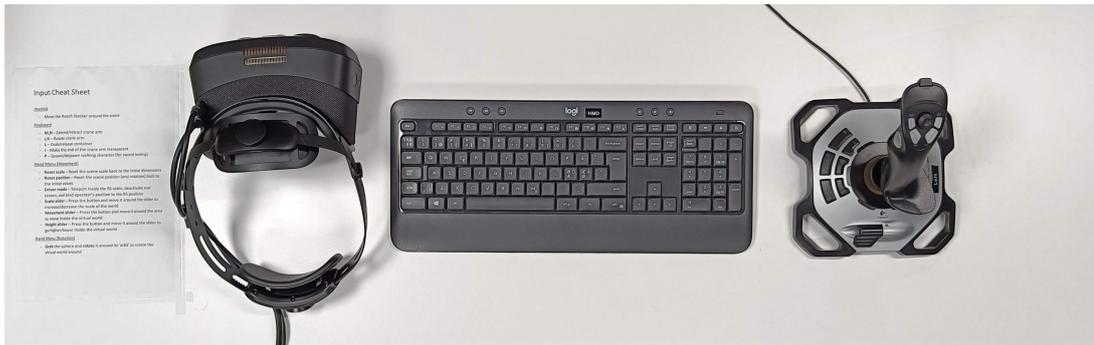
Figure 3.2: The first iteration of the application makes use of the keyboard to control the movements of the boom and spreader, and the joystick to control the reach stacker’s movement. A printed paper on the left summarizes all the controls available to the user, and they are divided into keyboard, joystick, and hand-tracking.
