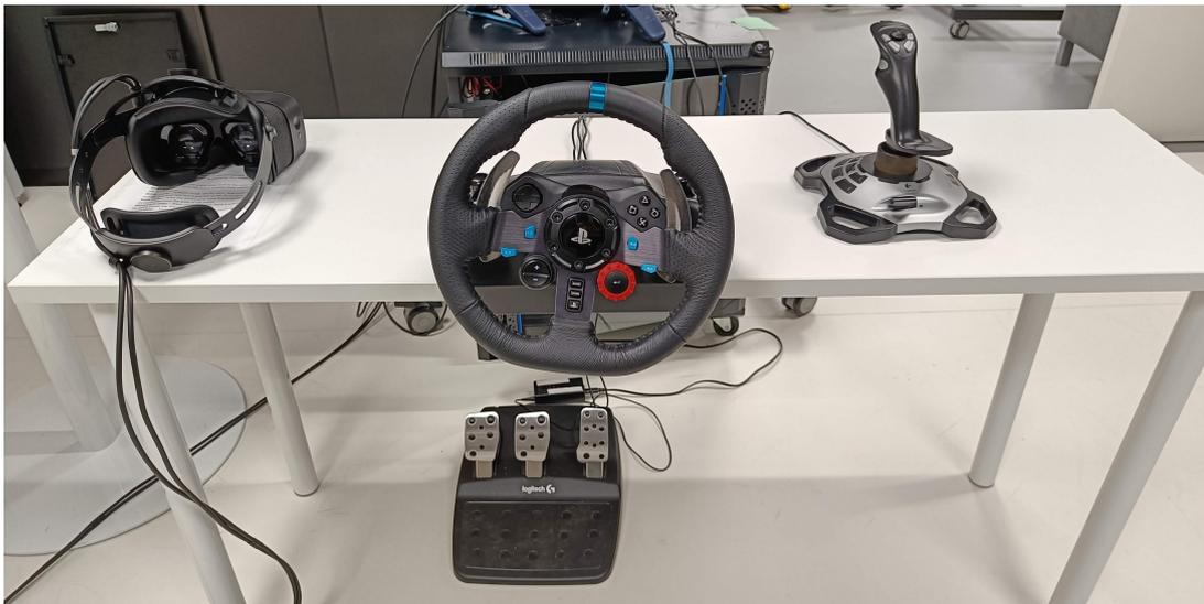
Figure 3.21: The second iteration makes use of a steering wheel and pedals, as vehicle movement is managed by a physical simulation. The keyboard is not needed anymore and the joystick now controls the boom and spreader, as the Logitech G29 is now used for driving. This setup is much more similar to the traditional reach stacker controls.
