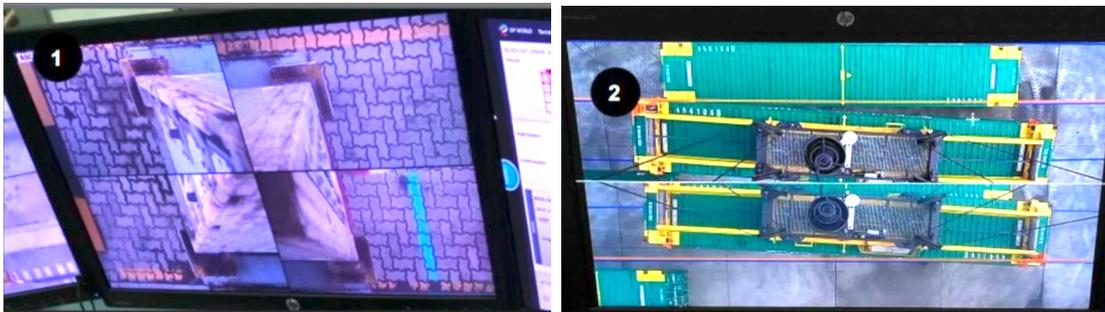
Figure 2.6: Operators need multiple cameras to correctly control the straddle carriers from a remote location.
