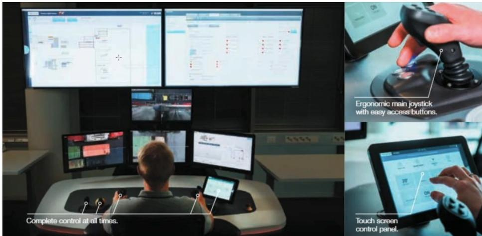
Figure 2.5: The current setup for straddle carriers' remote control.
