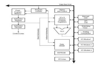
Fig5 Block Diagram System Architecture
