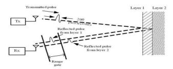
Fig4 A range gate at receiver
