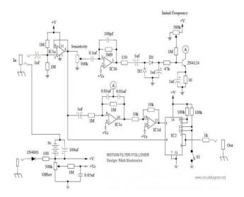
Fig 7 Circuit diagram for Motion filter
